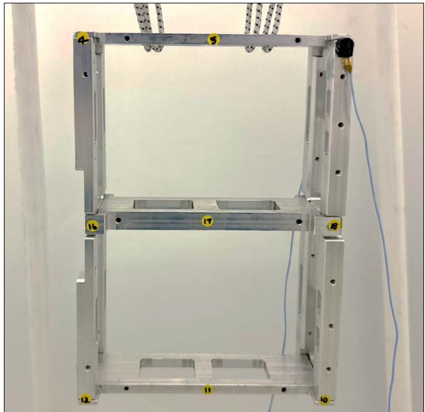
Figure 1. Hammer Impact Modal Test of the Satellite Model
