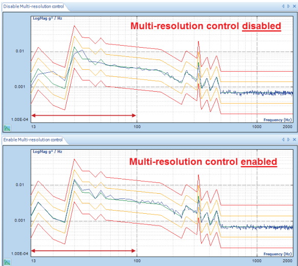
Compare control(f) with Multi-resolution control disabled and enabled. (profile range: 13~2000Hz)
