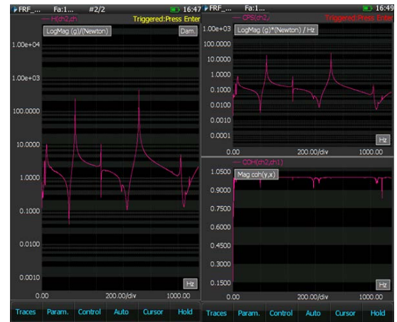
Figure 30. FRF, CPS and COH signals on CoCo
