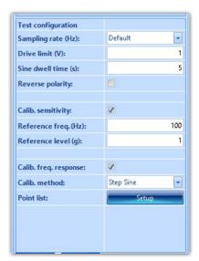
• Configurable profile for Swept Sine FRF measurement
