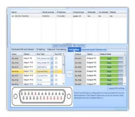
EDM 8.1 introduced a feature included in all the software modules including Vibration Controller and Dynamic Signal Analysis software. Users now have the ability to assign a specific test to each digital input. When the input is received, the test automatically runs.
