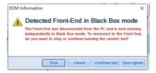
This new feature provides users the ability to Save Signals, which enables users to create a report at a convenient later time or to continue re-establishing a broken connection to view live signals.
