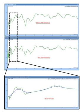
The zoomed in comparison of the overlapped FRFs shows that with the multi-resolution spectrum the peaks are much sharper and better identified as compared to it being flat without the enabled multi-resolution spectrum. The richer information is available because the finer resolution captures more peaks that are not as clearly visible and spread out in the normal spectrum.
