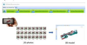
This feature utilizes the advanced technology of 2D to 3D reconstruction to provide a simple solution for the challenges of creating 3D geometric models from convoluted test structures. The imported images are matched to extract the features and a 3D model of the structure is constructed after the point and surface reconstruction processes are completed. This approach not only saves time and effort for the user, it also provides an accurate model with great simplicity.
