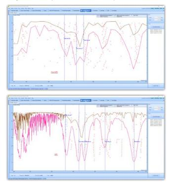
The stability diagrams above shows that the poles (frequency and damping) recognized with Multi-Resolution spectrum are more accurate because of finer frequency resolution.
