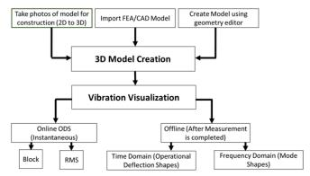
Building a 3D model of any structure is vastly simplified with the introduction of this feature. Any camera, including a cellular phone camera, can be used to capture images of an object from various angles to produce a 3D model of the structure.
