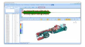
When used in combination with the vibration visualization feature of EDM software, animations representing a test object vibration on a shaker can be visualized.
