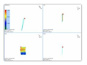
The scaling feature which uses the response data of the reference point has been added. Multiple references can now be executed with this OMA test module. Finally, a new modal parameter estimation method called the Stochastic Subspace Identification (SSI) is added. This dedicated curve fitting method for OMA is not only cleaner but more efficient as well.
