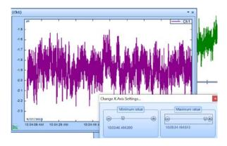
The sampling rates of these tests are typically under 100 Hz. Time Data Acquisition (TDA) software is equipped with the ability to save these raw time stream signals to the PC when the sampling rate is under 100 Hz. Users can choose a display option called "Time History" that allows the X axis of these signals to increase infinitely, resulting in a live view of the raw time signal for the entire duration of the test. Users can choose to view a smaller duration of live or historical data.
