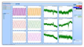
TDA is designed to be a lightweight software application targeting projects that only require time data acquisition without the need for additional processing.
