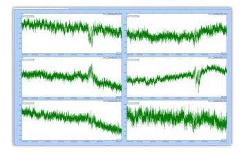
Users can save raw time recordings to the internal flash memory, allowing users to operate the Spider system in Black Box mode without an attached PC if necessary. Users can also save the low sampling rate raw time signals to the PC storage space for instant viewing without waiting for the test to stop.
