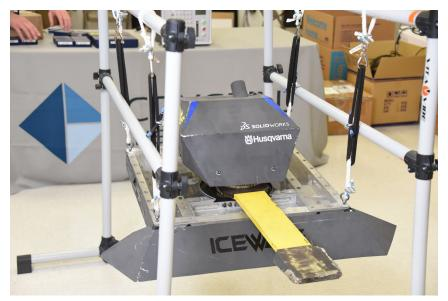
Figure 1: Icewave Bot Suspended in Modal Test Frame
